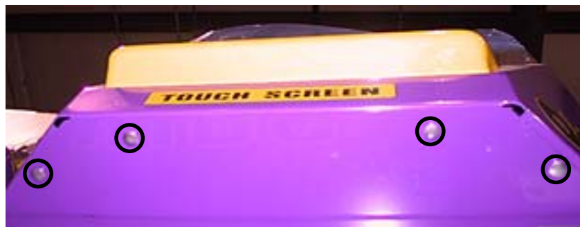
FIGURE 3 - FRONT OF SHROUD FASTENED WITH BOLTS
