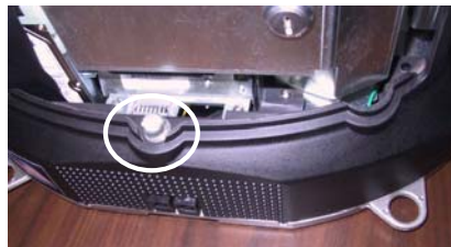
FIGURE 2 - SCREW IN CENTER OF BOTTOM COVER
