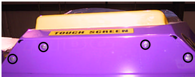
FIGURE 23 - FRONT OF SHROUD FASTENED WITH BOLTS
