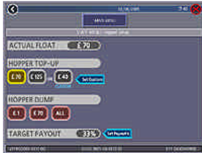
FIGURE 16 - S.W.P. MENU: HOPPER SETUP SCREEN
